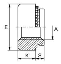
Female thread A = M3Height K = 2.0Max recess height = 1.0 Min distance to edge = 4.0Outer diameter E = 7.0
